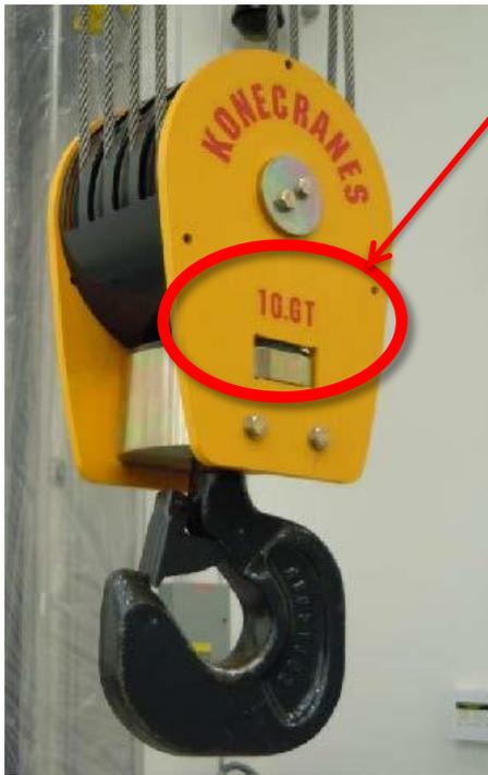
Load Markings are posted on all sides of the crane and on the hoist block.
