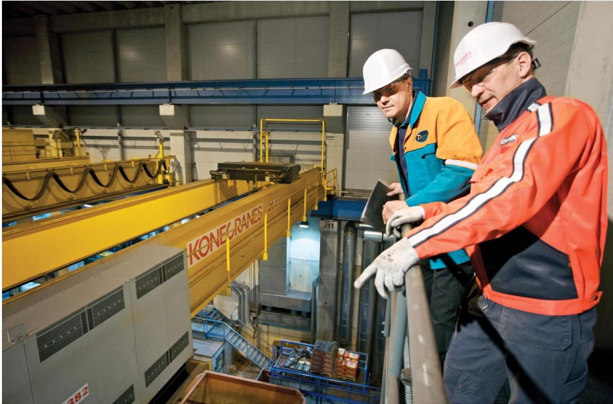
*While inspections are visual assessments of the crane and equipment, tests examine the operation and function of the machine.*
