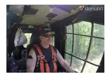
Use of a 5-point harness was advantageous to a traditional lap belt when properly adjusted to the shoulders. Reduced the total back & shoulder risk value by 50%
