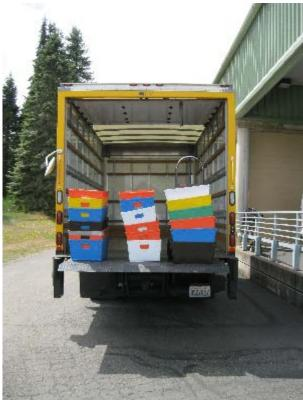
The use of a lift gate would have the most positive impact on reducing the risk factors of potential back injury. Considering the cost of equipping the TRL fleet, a smaller box van with a ramp would provide the same benefit as the vehicle rented for the test; this would be more practical for parking in narrow stalls and under covered parking areas.
