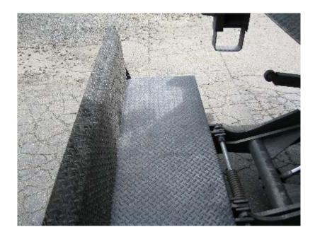
Even with the two piece lift gate, the advantage was evident; bending to lift boxes in and out of the vehicles was no longer required. Stacks of boxes were easily moved in and out of the vehicle with a hand truck. Up to 400 bends and lifts on the busiest route for just one day are eliminated with a lift gate, and up to 1300 per week for each of the six couriers.
