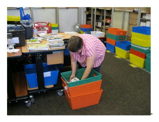
The HYDRA-2 model enables the sorters to consistently sort from the boxes at waist height, their "power zone" or at any desirable height.
