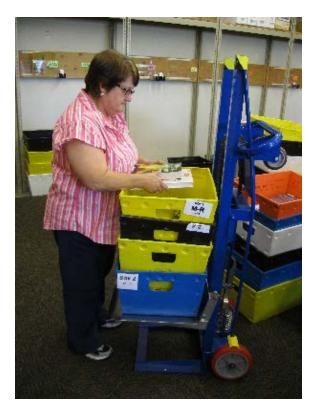
This is accomplished by pumping the hydraulic cylinder with one's foot.
