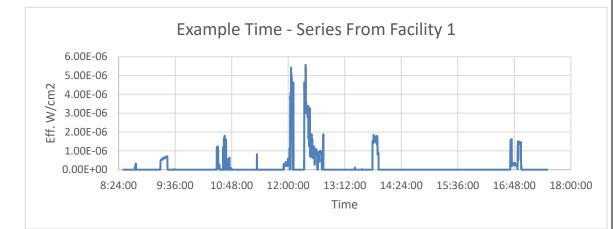
This figure illustrates a data time series recorded using the personal dosimeter on a worker at an indoor cannabis cultivation facility. The time series illustrates several "spikes" in UV exposure, several of which correspond to when the worker was outside - for example the major spikes between 12:00and 13:00 occurred when the worker took their lunch break outside.
