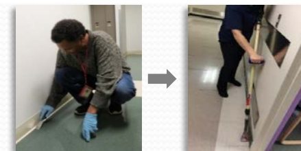
Modification: Long-handled scraper reduces crouching or flexion
