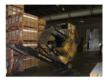
Ask the group what could have happened in this picture. Did you notice how all four tires are off the floor and the forklift is sitting on the main mast? The forklift was overloaded; the operator tried to back up and turn with the load raised. The next slide will show you what happened.
