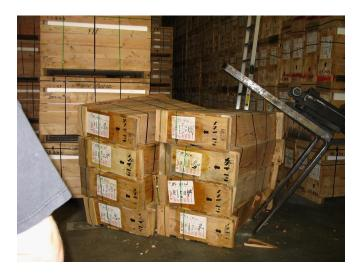
This forklift was over capacity. The operator raised the load, backed up and turned at the same time. The center of gravity moved outside of the stability triangle and the forklift tipped over.
