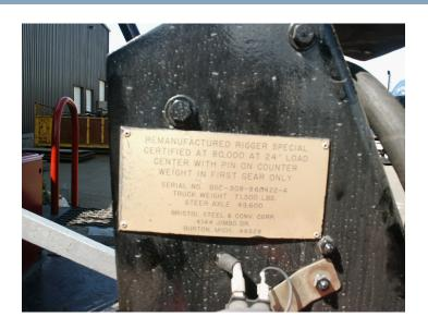
Read the information on the data plate. This forklift is a remanufactured rigger special. This forklift can lift 80,000 lbs. at 24 inch load center in first gear only.
