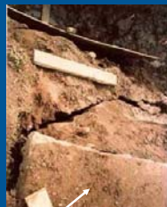
This soil is fissured changing the classification from A to B
