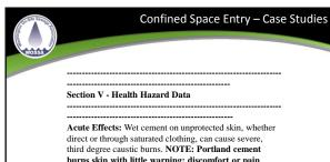
burns skin with little warning; disconfort or pain cannot be relied upon to alert a person to a hazardous skin exposure. The severity of the burn may not be detected until several hours after the damage begins. Dry portland cement can produce mild irritation to severe burns of the eye; it can irritate the upper respiratory system.
