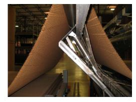
worst case (4 inch, type 1 core) on a partial rack, as opposed to the optimum configuration where the core flake is at the same level as the roll which virtually eliminates any lifting and significantly reduces the grip force to transfer the flake across the roll. Results are below.
