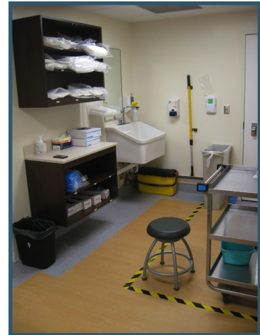
Ante room showing well-marked dirty/clean floor delineation, seat for changing into clean and out of dirty areas, sink and hand sanitizing station, and gown and glove storage area.
