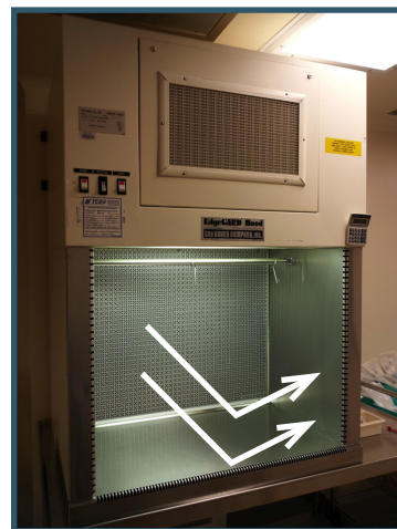
Laminar flow hoods are not appropriate for preparing and manipulating hazardous drugs because the air flow is toward the preparer.
