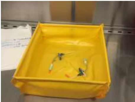
Photo 3: Typical air sampling set-up during a spill condition (Phase 1/Phase 2)
